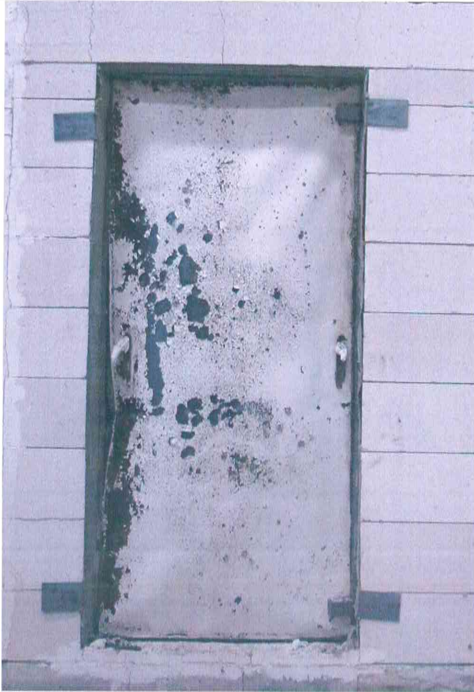
Figure C4: Exposed side of the test specimen after the test.
