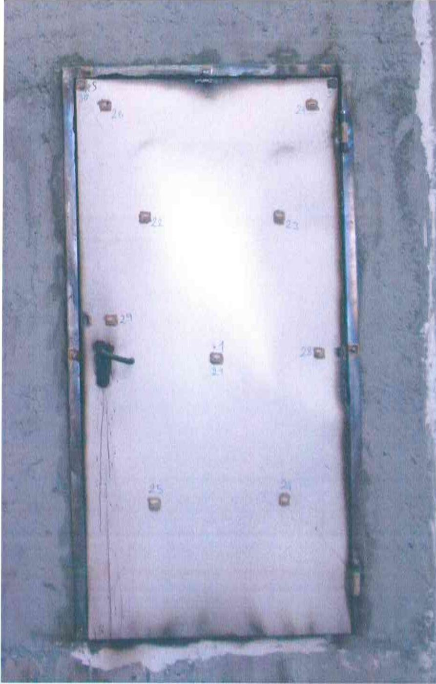
Figure C3: Unexposed side of the test specimen after the test.
